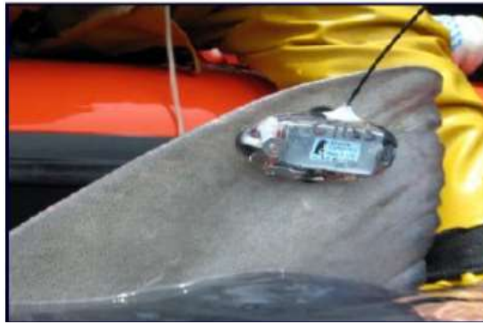
Figure 4: SPOT tag attached to the dorsal fin of a tiger shark
