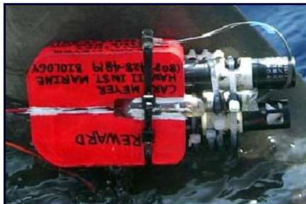
Figure 7: Accelerometer datalogger and digital camera deployed on a tiger shark
